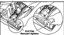
After checking the end caps, reinstall the agitator brush assembly back into the housing grooves After installing the agitator brush assembly, turn it by hand making sure that the belt is not twisted and all rotating parts turn freely. Replace the lower plate as described in the Removing/Installing the Lower Plate section
