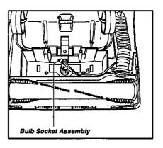
4 Reinsert the bulb socket into the nozzle housing by pushing it back down into the slot Replace the lower plate as outlined in the Removing/Installing the Lower Plate section
