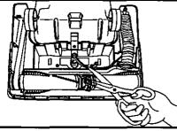
Switch off the vacuum cleaner and unplug the power cord before cleaning the agitator assembly In order to keep the cleaning efficiency high, clean the agitator assembly regularly Remove the lower plate if necessary See the Removing/Installing the Lower Plate section for the proper procedure
